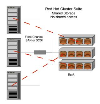
Shared physical storage Each server mounts Ext3 disk partitions privately Failover allows different server to remount partition after failure
